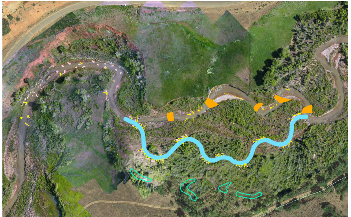
Preliminary design for proposed channel enhancement work includes: adding woody debris to the main channel (yellow), adding boulders to the main channel (pink), rerouting the main channel in an area with eroding banks (light blue), creating check dams (orange) in the abandoned channel to form ponded habitat, and excavating new ponded habitat (green outlines).
