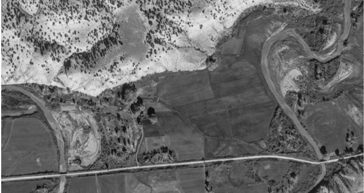
Figure 5.2. Magnified image of black rectangle shown in Figure 5.1. Despite significant development of the valley bottom for agriculture, the river shows localized areas where the active channel is approximately 5-10x the width of the low-flow channel, and there is evidence of significant areas of bare alluvium.
