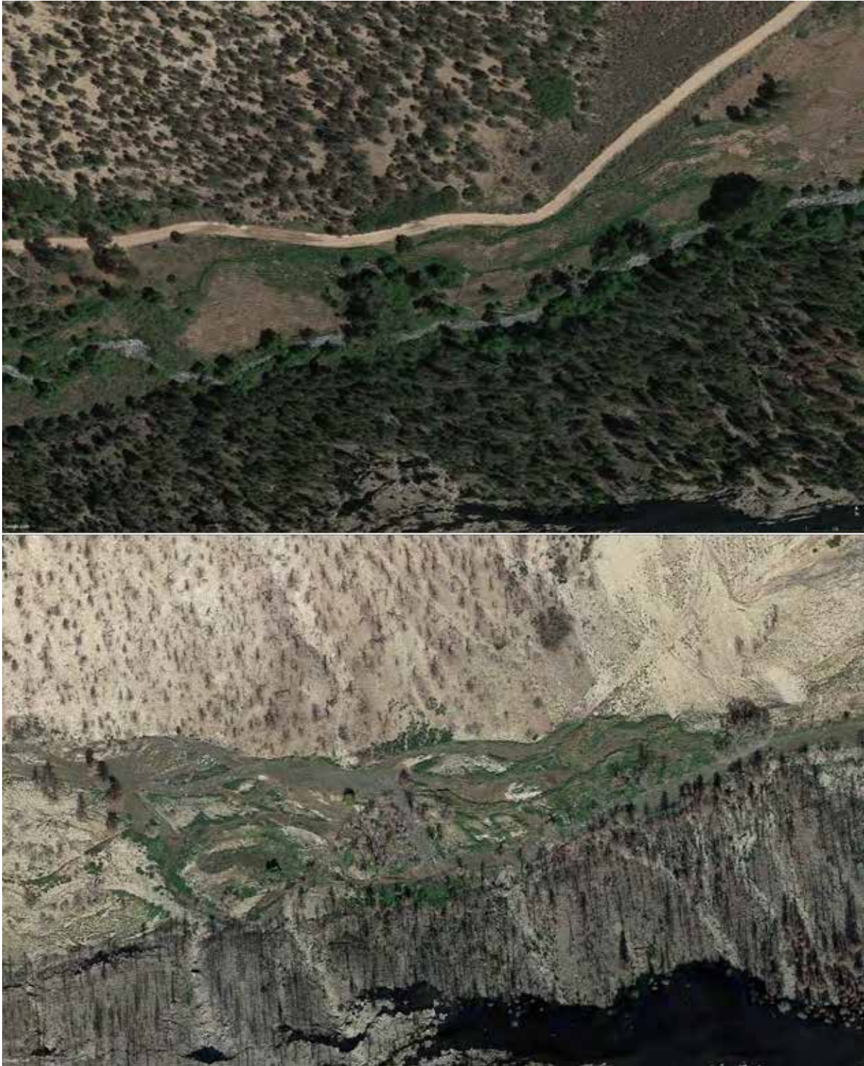
Figure 5.3. Pre- and post-fire on the Strawberry River immediately below Sulfur Draw (river Km 18). Assessing both pre- and post-fire conditions is critical to understanding the impact of post-fire changes and assessing recovery trajectory and potential. Flow is from left to right.
