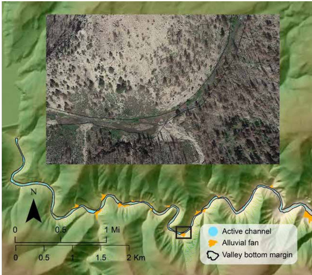
Figure 4.5. Reach 1 is confined with floodplain pockets. Hillslopes are the most important confining margin, though small alluvial fans are present.
