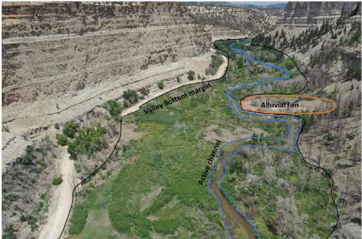
Figure 2.5. Illustration of valley bottom and active channel delineation near river kilometer 29, roughly 1 km upstream of Pinnacles.
