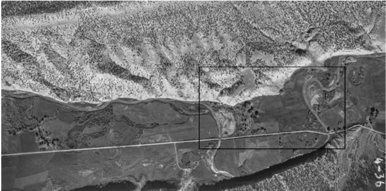
Figure 5.1. 1961 aerial imagery of the Strawberry River downstream of Pinnacles. While outside of the project area, this image illustrates that in wide valley bottoms the Strawberry River was historically characterized by a wider active channel with exposed alluvium. By 1961, flow regulation had already been present for 50 years, but was not yet as affected as it would be following the construction of Soldier Creek dam in 1973. The black rectangle shows the extent of the magnified image shown in Figure 5.2.
