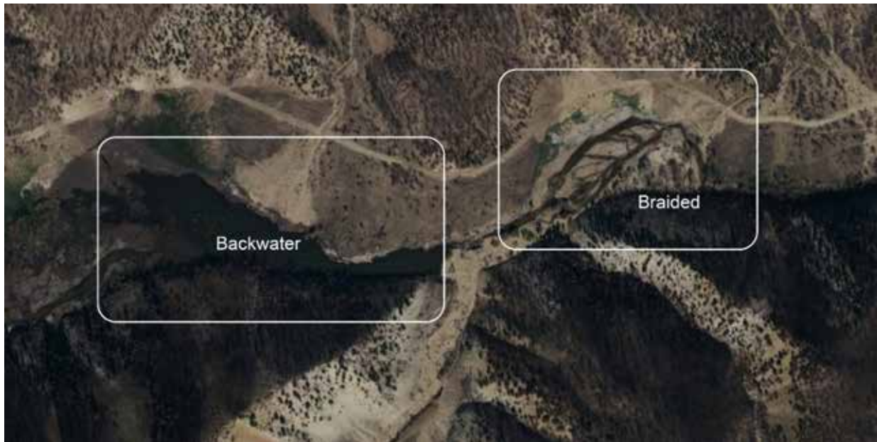
Figure 2.8. Aerial imagery of Slab Lake, an extensive backwater forced by the damming of the Strawberry River that resulted from sediment delivered from Slab Canyon. Downstream, the Strawberry river exhibits a braided planform, likely the result the same high sediment supply that forced the upstream backwater. Throughout the project area, backwaters and braided, and multi-channeled planforms were common post-fire. These areas represent some of the most complex habitat on the Strawberry River, and are forms that were not present pre-fire. Given limited snowmelt-driven peak flows, features such as Slab Lake are likely to persist for a significant amount of time. Braided planforms will likely transition to either multi-channeled planforms, if vegetation stabilizes current bars, or single-thread channels.
