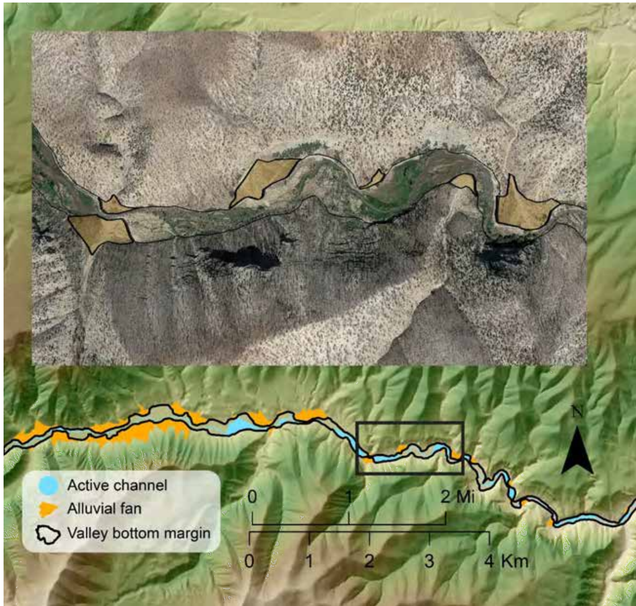
Figure 4.7. Reach 3 is characterized by extensive influence of intermittent tributary junctions that have caused major changes post fire, including backwaters, and braided and multi-threaded channels which have produced a much wider active channel.
