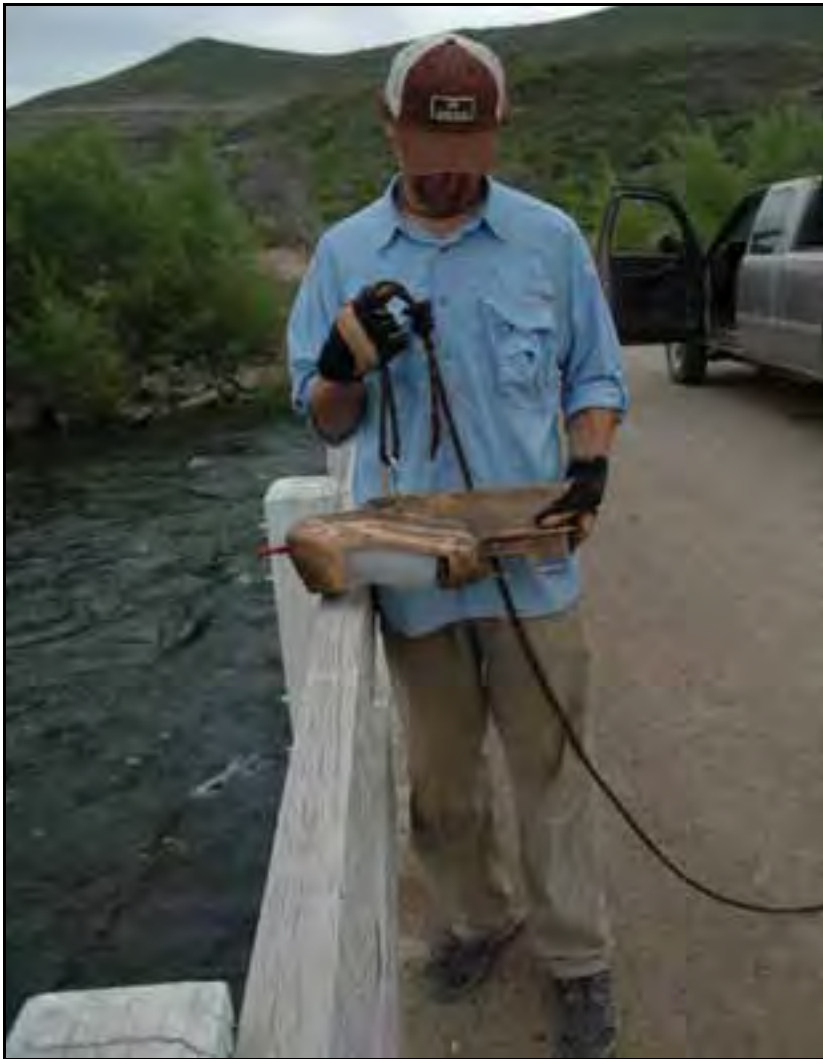
Photo 4.2. Depth-integrated hand line type model US DH-76 suspended sediment sampler.
