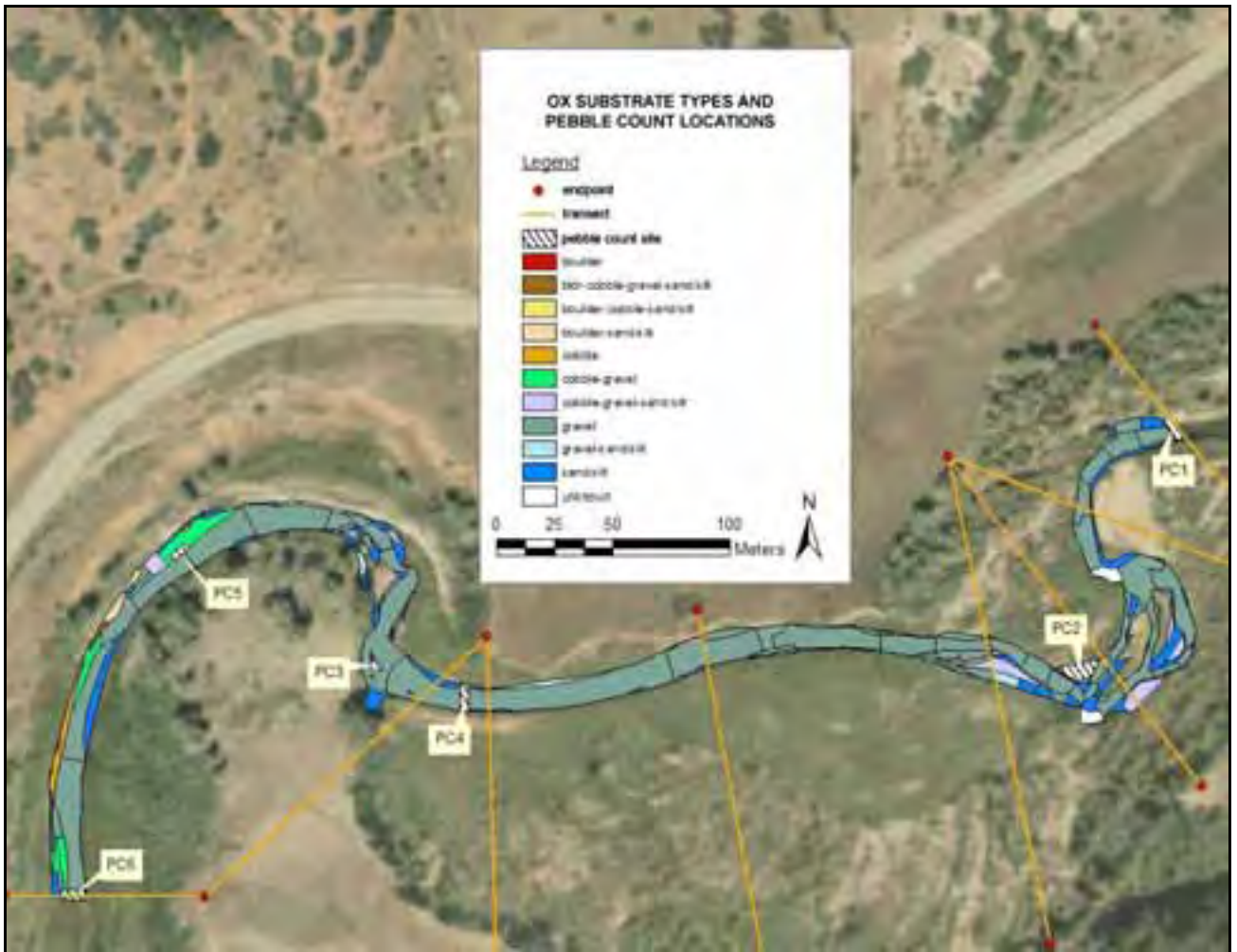
Figure 3.1d. Major substrate types and pebble count patch locations at the Oxbow (OX) monitoring site. Aerial photo from 2006.
