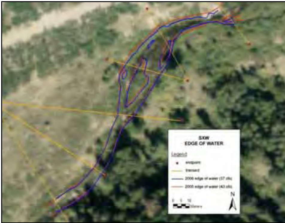
Figure 2.6. Location of the surveyed edge of water at the Sixth Water (SXW) site in 2005 (43 cfs) compared with 2006 (37 cfs). Aerial photograph from 2006.
