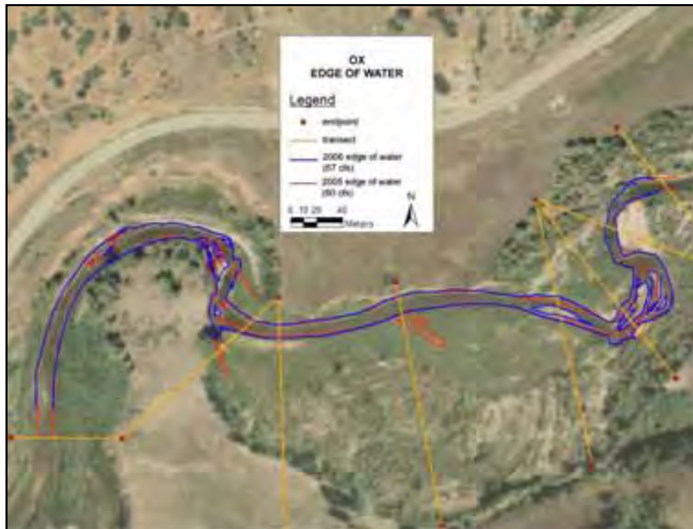
Figure 2.9. Location of the surveyed edge of water at the Oxbow (OX) site in 2005 (60 cfs) compared with 2006 (67 cfs). Aerial photograph from 2006.
