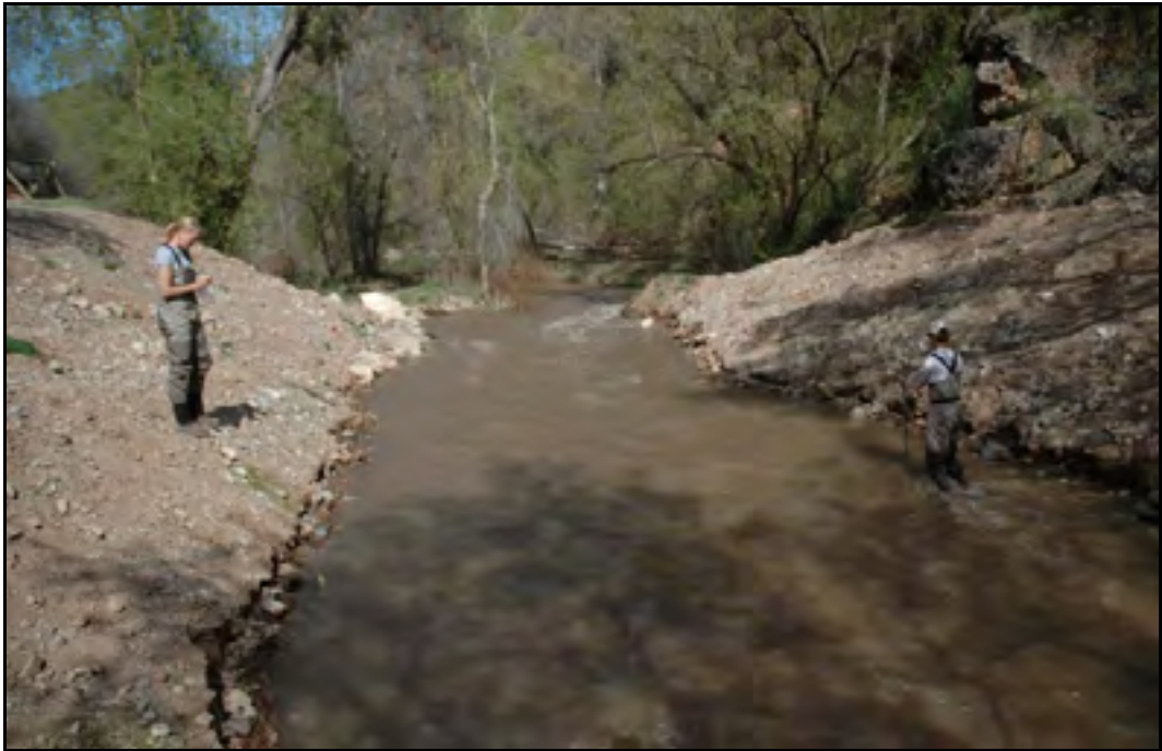
Photo 4.3. Bedload sampling using the 3-inch hand-held sampler. Photo taken at the Diamond Fork above Three Forks monitoring site.
