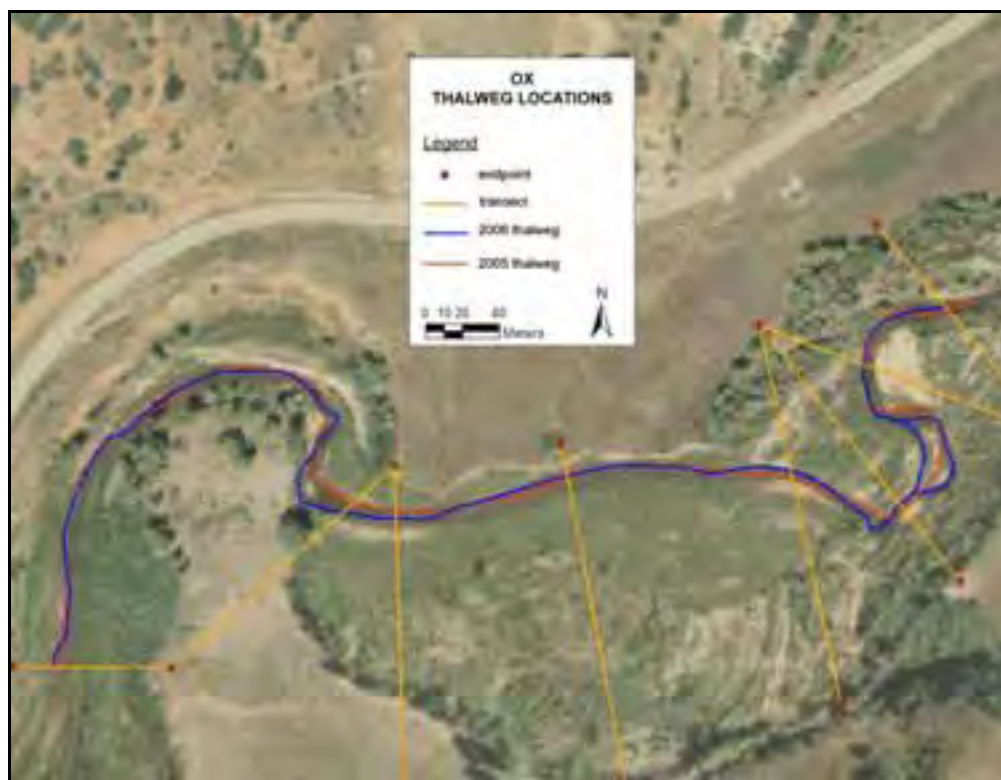
Figure 2.13. Location of the surveyed thalweg at the Oxbow (OX) site in 2005 compared with 2006.
