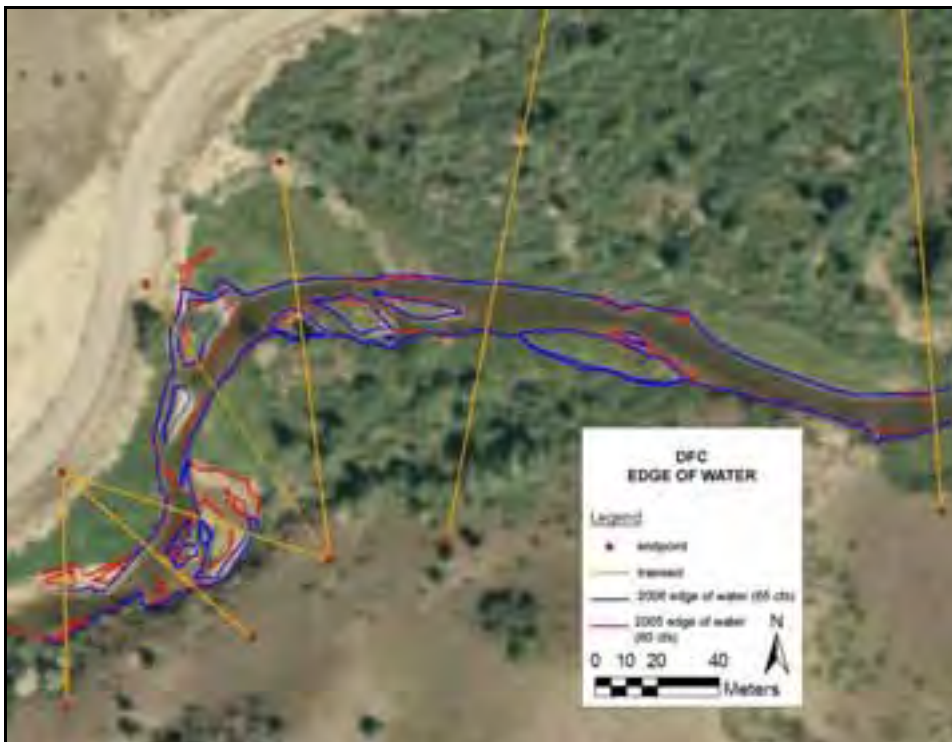
Figure 2.7. Location of the surveyed water edge at the Diamond Fork Campground (DFC) site in 2005 (60 cfs) compared with 2006 (65 cfs). Aerial photograph from 2006.
