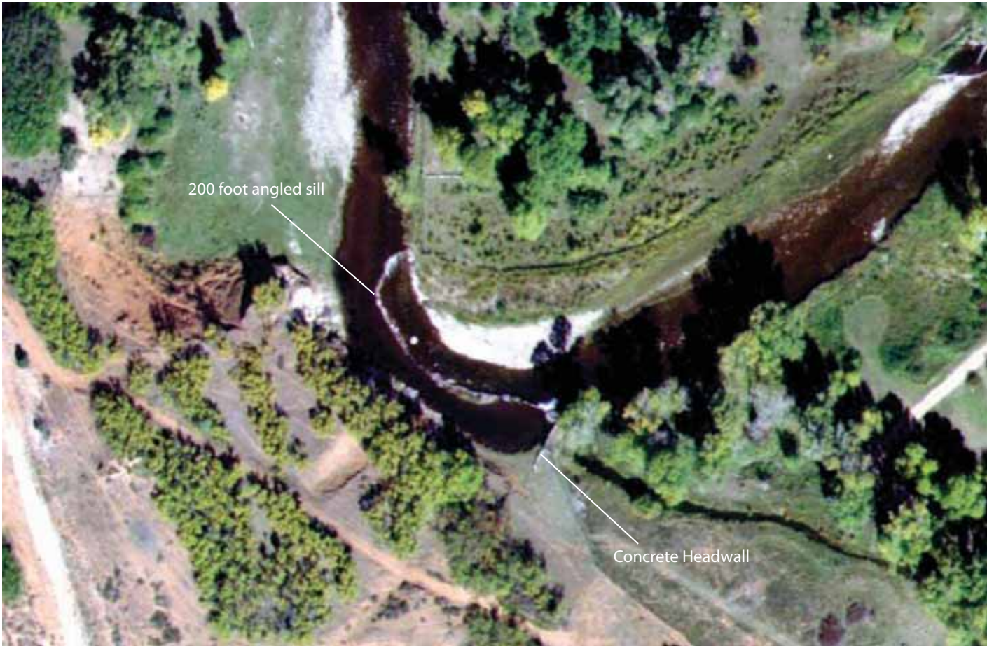
Figure 3. Aerial image of the pre-project condition of the Duchesne River at the Turnbow Diversion, showing the long angled sill and the location of the headwall.
